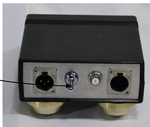
GEM silver controller rear panel, power plug left, main servo motor power switch motor plug on the right. The main power provides electrical platter breaking and is left on most of the time
