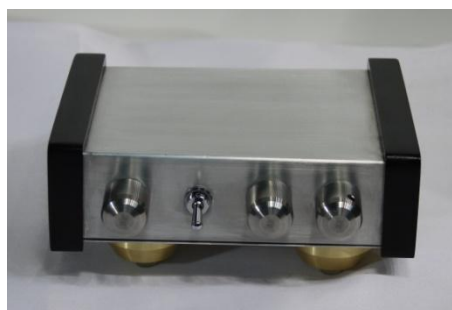
GEM ultra controller, front panel, left is 33/45 speed selector, middle platter on/off, two controls on right, pitch for 33 and pitch for 45 rpm
